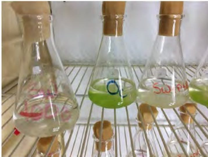
Photo 3: From left to right, site water without nutrients, lab water control, and site water + N and + P on Day 5
